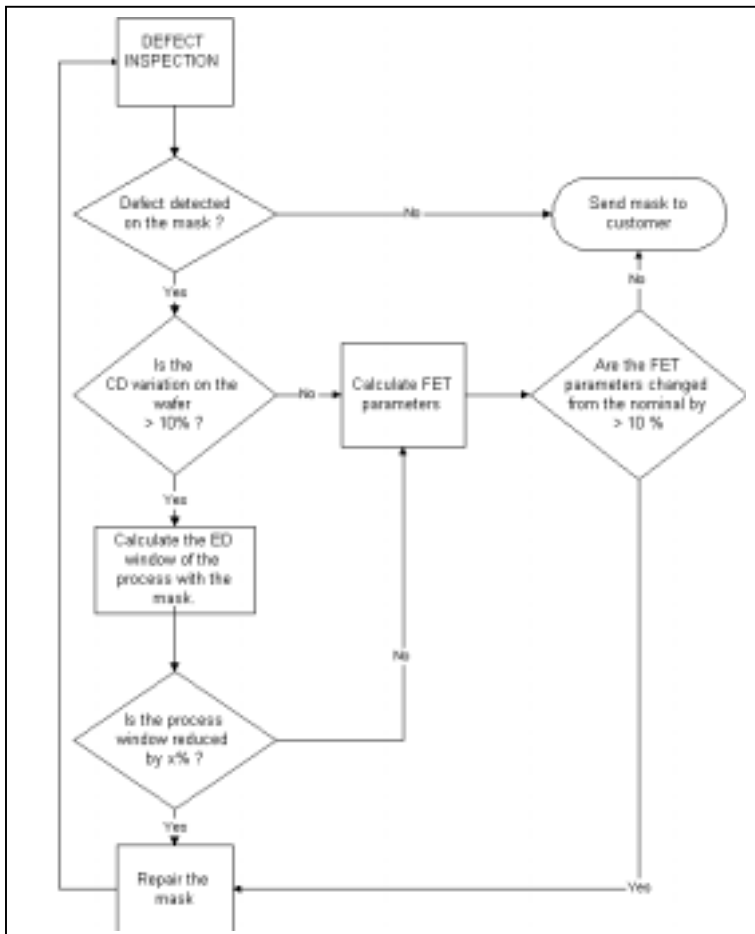
Figure 2: The novel mask qualification procedure proposed in this work. In addition to the disposition criteria proposed in Fig.1, it would also involve an additional one – the allowed change of MOSFET parameters (here, by 10\% ).
