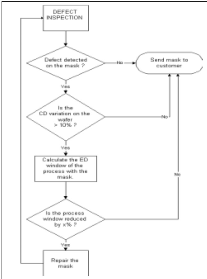
Figure 1: An example of advanced procedure to qualify mask defects and disposition of critical mask layers using simulation of silicon image. An important parameter is the allowed process window reduction ( x\% ). Process window calculation is based on the exposure/defocus matrix simulated based on the mask.
